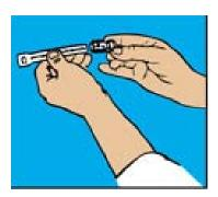
WRAPPED ONCE AROUND Insert end of rack into housing and turn screw just enough to engage rack. Be sure words "THIS SIDE UP" on rack are facing operator.
