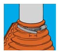
Insert hook into other band blot, and flatten with thumb forming clamp. Tighten screw with screwdriver to desired tension. Clamp is complete.
