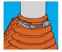
Bend end of band toward underside to form hook and insert in band slot on housing. Wrap the assembly snugly around object and at point ONE INCH BEYOND first serration, cut, then bend a 1" hook toward underside of band.
